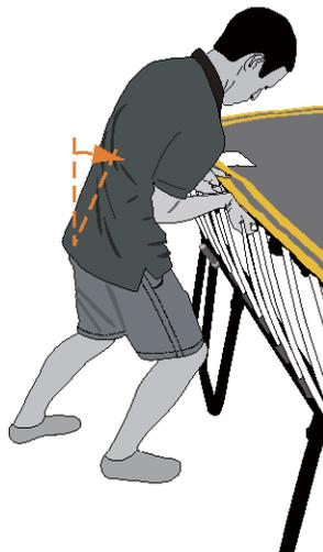
3 Push forward rocking from your heels to the balls of your feet, using the weight of your body to push the white mat rod into the mat rod holder while you keep the mat edge horizontal with your other hand
