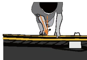
4 Pushing across your body in the direction shown will make it easier to get the mat rods in or out of the mat rod holders.
